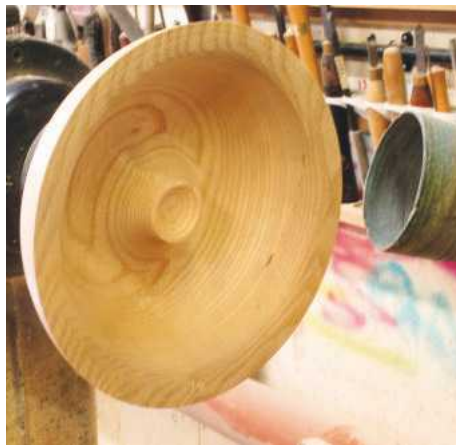
▲ Pic.14 The inside bowl turning is complete. The centre stem must be tall enough to put the nut on easily but if it's too high the shells can fly out during the hammering process
